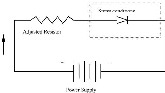
Figure 3. Adjustable Resistor and LEDs Circuit
