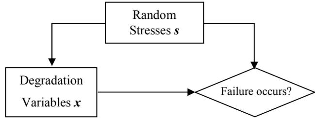
Figure 1. Both degradation process and random stress affect the likelihood of the occurrence of a failure.
