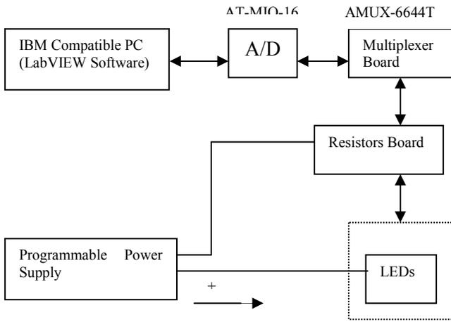
Figure 2. The Layout of Experimental Equipment
