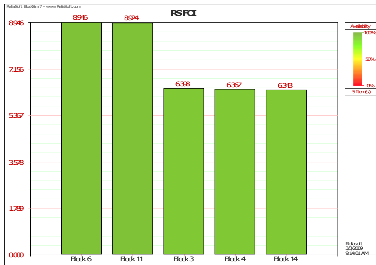
Figure 6: Failure criticality indices obtained with BlockSim 7
