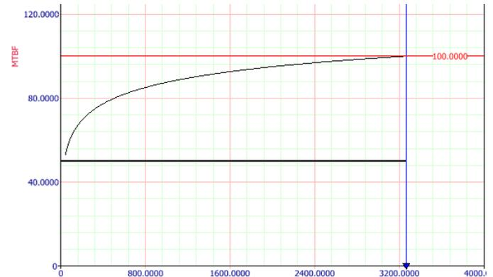
Figure 2: Extended Reliability Growth Model Planned Curve
